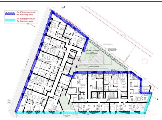
Figure 5: Glazing mark up Level 3-6
