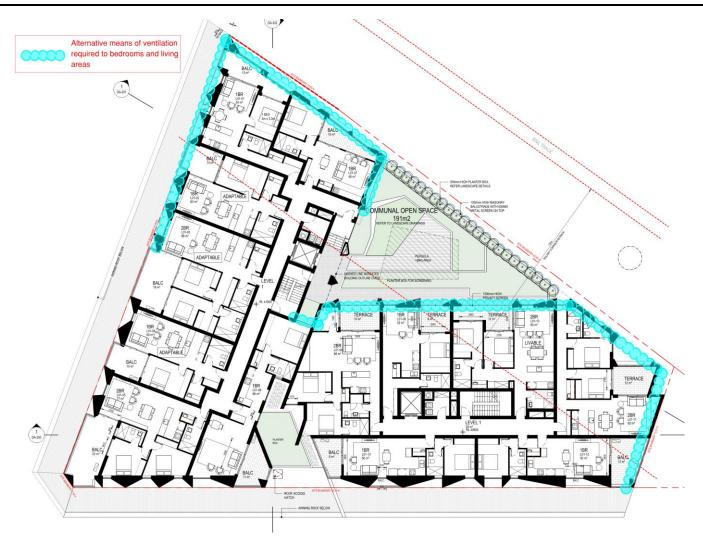
Figure 9: Alternative ventilation mark-up (typical for levels 3 - 6)
