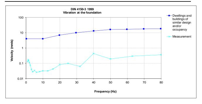
Based on the measured vibration levels at the façade of the proposed development, it is not expected that there will be any exceedance of the criteria established with regards to structural damage. There is also no exceedance of the VDV criteria for human comfort during the day or night time.
